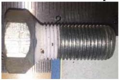
Now is a good time to test fit the spacer to the Axle & then to the wheel rim. The spacer should make full contact to the axle & the nuts/lug bolt has full tread contact , it's much easier to sort any problems without having anything bolted down.
